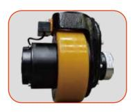
Adopt 1.3KW AC horizontal drive and equipped with 250x80 drive wheel ensure stronger carrying capacity; high power and accelerated stability, low maintenance cost as no need to replace the carbon brush; good ramp starting performance. Both sides are equipped with spring regulating structure stability castors ensure better wear resistance and stability.
